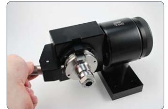
The tool holder will snap in automatically. To release pull out on the release pin
